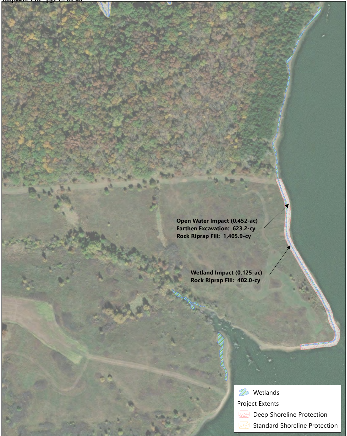
Figure 2G. Plan View Request for Individual Permit Three Mile Lake Restoration Project Iowa Department of Natural Resources
